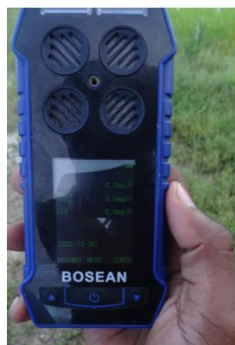
▪ Plate 1.5 (b): Gas Detector for SO 2 , NO 2 , O 3
