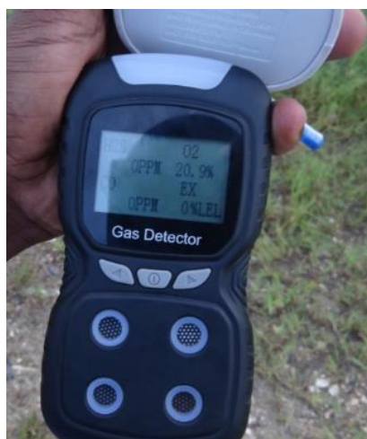
▪ Plate 1.5 (a): Gas Detector for O 2 , H 2 S, CO, Combustible Gas
