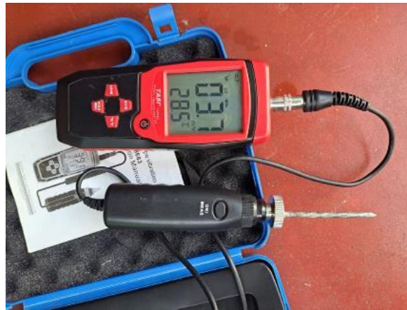
Plate 1.6: Vibration Meter used in this study (Photos were taken during field work for this ESIA study between October and December, 2022)
