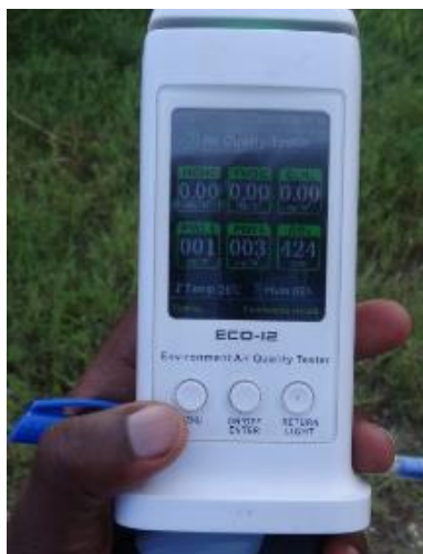
Plate 1.4: Environmental Air Quality Tester (Photos were taken during field work for this ESIA study between October and December, 2022)
