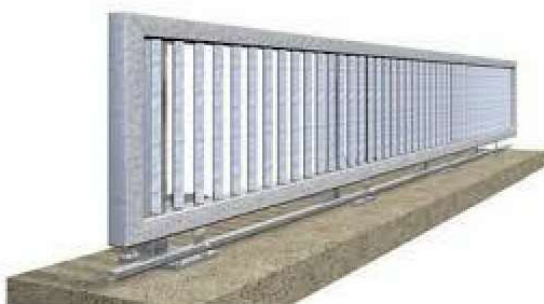
Figure 2-4: Typical Illustration of Metal Parapet Systems
