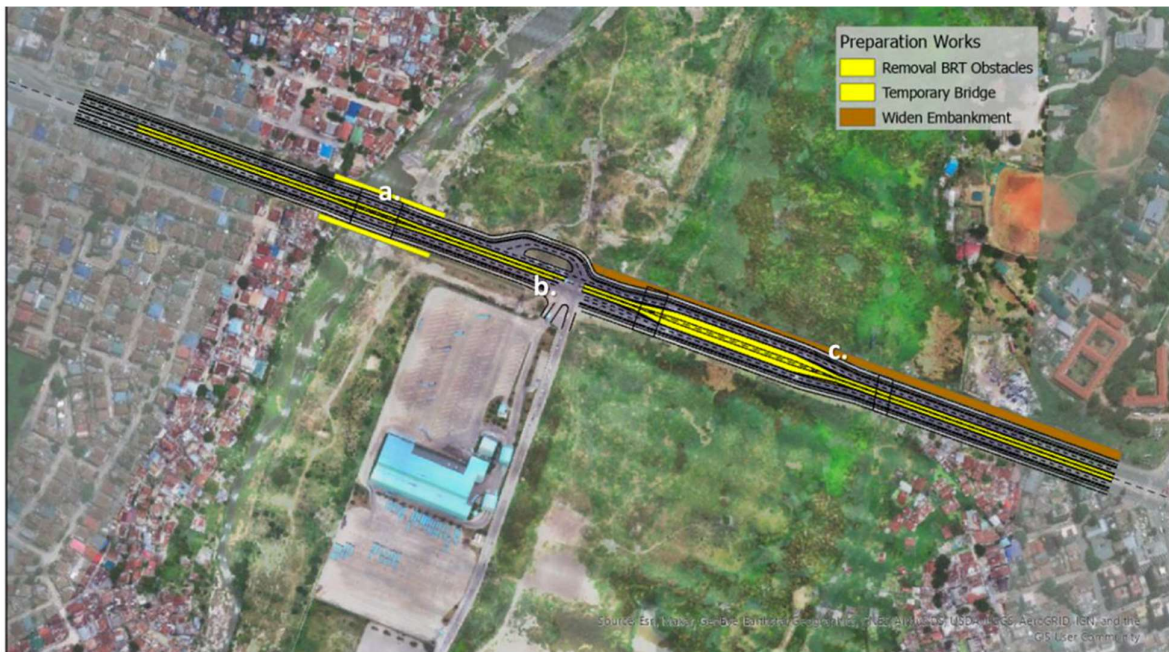
Figure 2-18: Schematization of preparation works for Temporary Traffic
